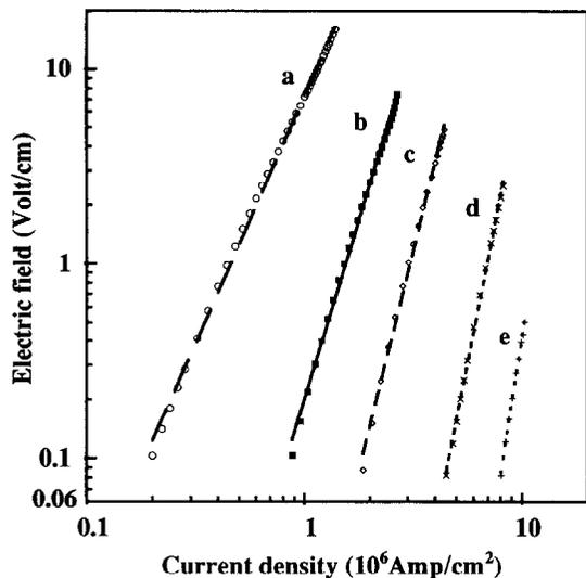
Fig. 6.  $I$ - $V$  curves for sample A in a 0.4 T magnetic field plotted as electric field vs. current density at (a) 85.90 K, (b) 80.96 K, (c) 76.07 K, (d) 65.96 K and (e) 55.92 K.
