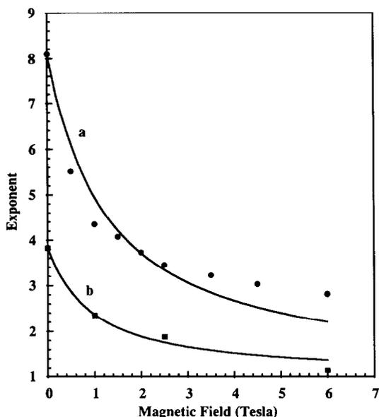
Fig. 9. Variation of the exponent with magnetic field at temperatures of (a) 80.61 K and (b) 86.01 K. Points indicate experimental data and the curves indicate the expected theoretical variation.
