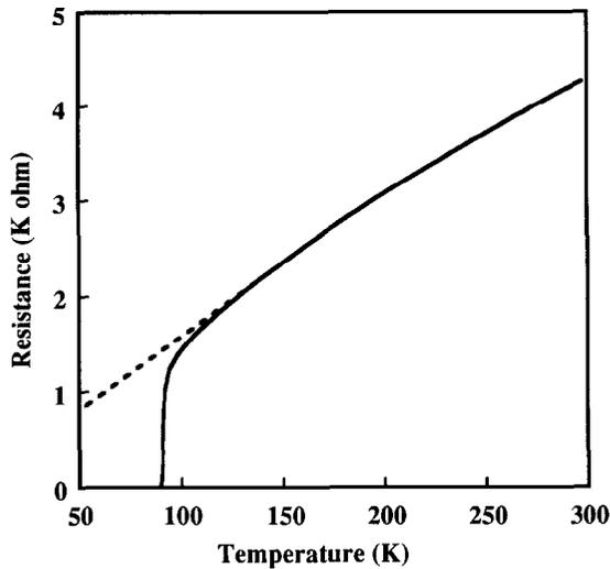
Fig. 2. Resistance vs. temperature plot for sample A. The dotted line indicates the extrapolated normal resistance at temperatures below the transition temperature.
