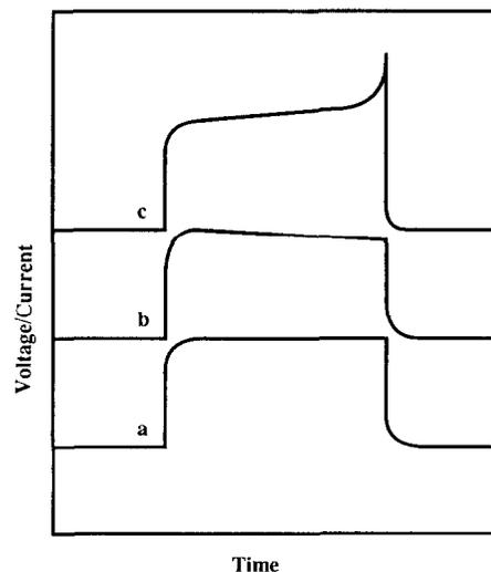
Fig. 4. Shape of the current and voltage pulses. (a) Current or voltage pulse at low power density and (b) current and (c) voltage pulses at high power density.
