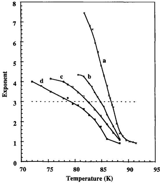
Fig. 8. Variation of the exponent with temperature for sample B in (a) zero field, and in magnetic fields of (b) 1.0 T, (c) 2.5 T and (d) 6.0 T. The dotted line indicates the value of the exponent expected at the K-T transition. Curves are plotted to guide the eye.
