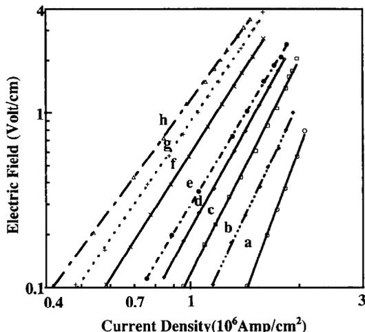
Fig. 7.  $I$ - $V$  curves for sample B plotted as electric field vs. current density at 80.61 K in magnetic fields of (a) 0.5 T, (b) 1.0 T, (c) 1.5 T, (d) 2.0 T, (e) 2.5 T, (f) 3.5 T, (g) 4.5 T and (h) 6.0 T.
