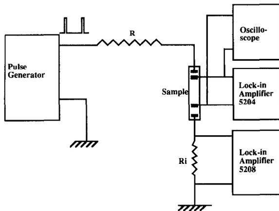
Fig. 3. Circuit diagram for pulse  $I$ - $V$  measurement.
