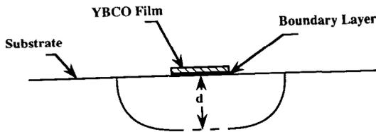
Fig. 1. Heat flow in the sample.
