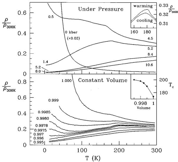
FIG. 2. Upper curves give the temperature-dependent resistivity of  $\text{RbC}_{60}$  at zero pressure and five clamping pressures. Numerical labels give the pressure in kbar at 4.2 K and 300 K. The inset shows the hysteresis in the 5.2 kbar clamping pressure data. The lower set of curves shows the constant-volume resistivity, labeled by the fraction of the  $(P, T) = (0, 0)$  volume occupied at  $T = 0$ . The inset shows the variation in the resistive feature with volume.
