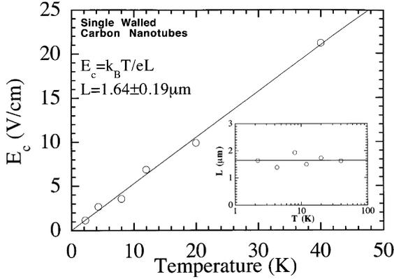
Fig. 3. The critical electric fields,  $E_c$ , shown in Fig. 2, is plotted as a function of temperature. The inset shows the localization length scale  $L$ , defined in the text, as a function of temperature. The line denotes the average value,  $1.64 \mu\text{m}$ .
