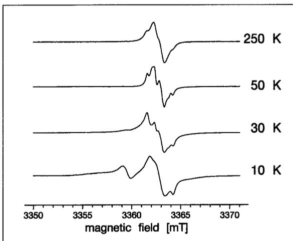
**FIGURE 2.**  $Rb_1C_{60}$  single crystal EPR signal for different temperatures at 94 GHz. At 50 K and above the signal exhibits an angular dependence that is not observed below the metal-to-insulator transition.
