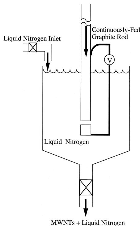
Fig. 1. Schematic of continuous production liquid-nitrogen reaction chamber for nanotube synthesis.
