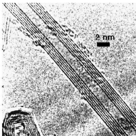
Fig. 2. High-resolution transmission electron microscope image of a multi-walled carbon nanotube produced by the liquid-nitrogen arc reaction method.
