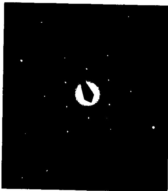
Figure 20.15 Electron diffraction pattern of C 36 crystallite. The pattern is hexagonal with a calculated d -spacing of 6.68 Å.
