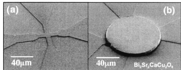
FIG. 1. Scanning electron microscope image of a GaAs/AlGaAs Hall sensor (a) with no sample and (b) with a BSCCO disk mounted on top of the Hall sensor. The sensor has an active area of  $10 \times 10 \mu\text{m}^2$ . The BSCCO disk has a diameter of 93  $\mu\text{m}$  and a thickness of 4.5  $\mu\text{m}$ .
