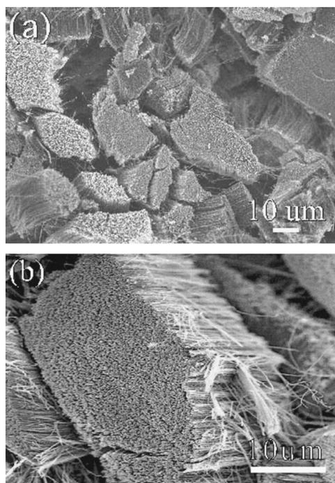
FIG. 1. (a) Low magnification SEM image showing a general view of the bundles of the aligned  $B_xC_yN_z$  nanotubes and (b) high magnification SEM micrograph revealing a high density of aligned nanotubes.
