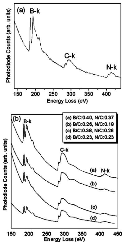
FIG. 3. (a) Typical EELS core electron  $K$ -shell spectrum taken from an individual nanotube of aligned  $B_xC_yN_z$  nanotubes and (b) a comparison of EELS spectra recorded from four locations along the nanotube indicated in Fig. 2(a).
