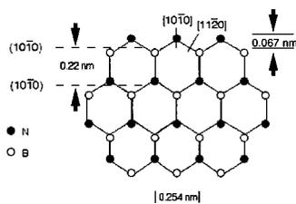
FIG. 2. Schematic sketch of boron nitride basal plane, showing the  $\{10\bar{1}0\}$  bilayers.
