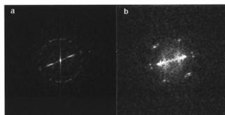
FIG. 3. FHT spectra of (a) Two-walled, (b) four-walled boron nitride nanotubes. Note orthogonal reflections in (a) and six-fold array in (b). Also note spacing difference in the  $(0002)$  reflections (innermost two maxima) between the two cases.
