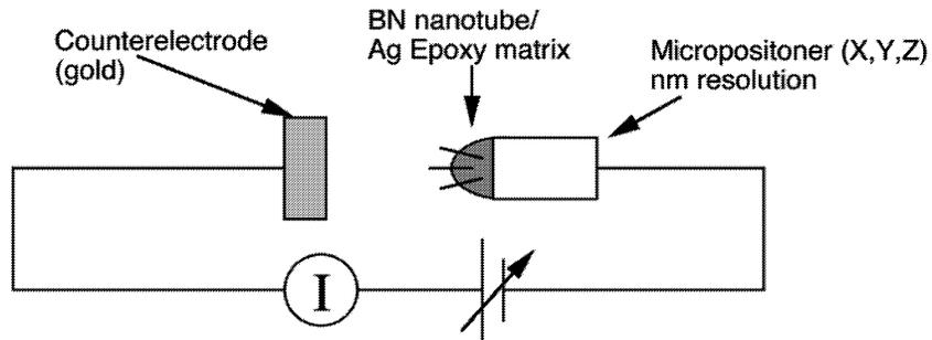
FIGURE 1. The experimental setup for electrical measurements inside the TEM.
