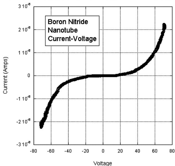
**FIGURE 3.** The current-voltage characteristic of a typical BN nanotube under contact conditions.
