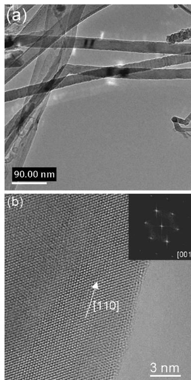
FIG. 1. (a) Low-magnification TEM image showing a general view of the GaN nanorods and the carbon nanotubes in the product and (b) high-magnification image of part of a nanorod. Inset is the corresponding diffraction patterns taken by FHT techniques. The incidence direction of the electron beam is along (001) direction.
