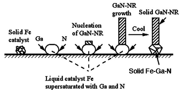
FIG. 3. Schematic illustration of VLS process for GaN nanorod (GaN-NR) growth by a pyrolysis route.
