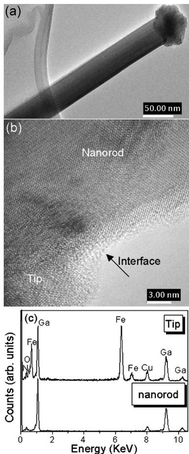
FIG. 2. (a) Low-magnification image of a GaN nanorod including its tip, (b) a high-magnification image of the interface of the tip and the nanorod, and (c) EDS spectra taken from the tip (upper) and nanorod (down), respectively.
