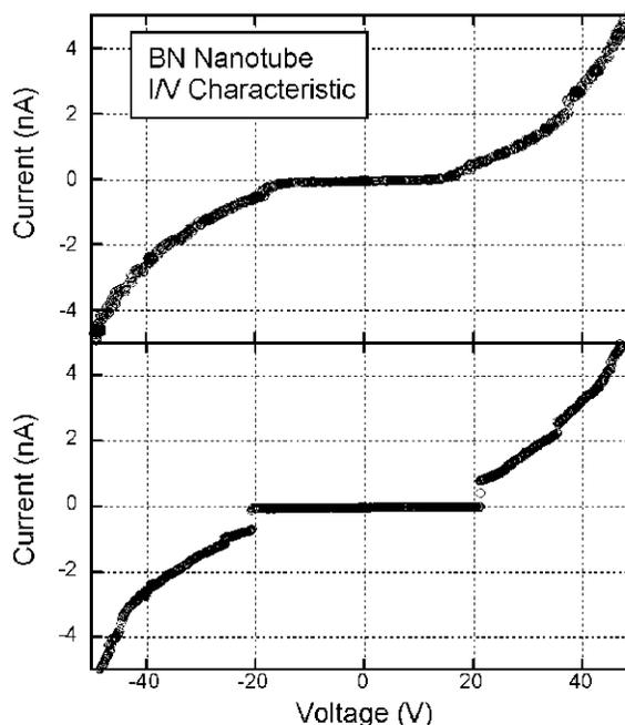
Fig. 3. The current-voltage characteristic of typical BN nanotubes under contact conditions. In both cases, the nanotubes protrude from the conducting matrix approximately 400 nm.
