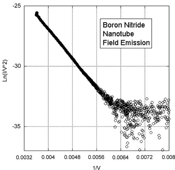
Fig. 2. Fowler–Nordheim plot of the current-voltage characteristic of field emitting BN nanotubes.
