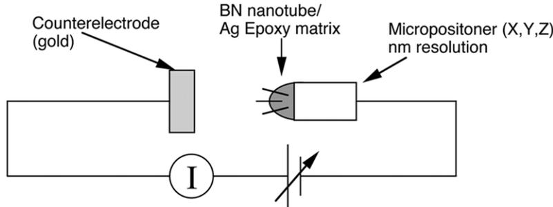
Fig. 1. The experimental setup for electrical measurements inside the TEM.
