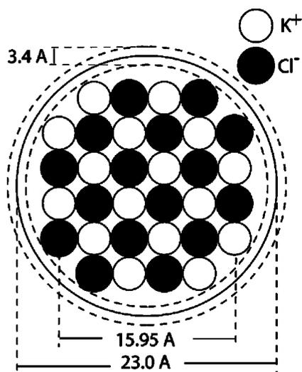
FIG. 2. Simulation image of the cross section of KCl-filled BNNT. In comparing this image to Fig. 1, the vertical direction ( $(100)$  axis) would be parallel to the imaging electron-beam direction.
