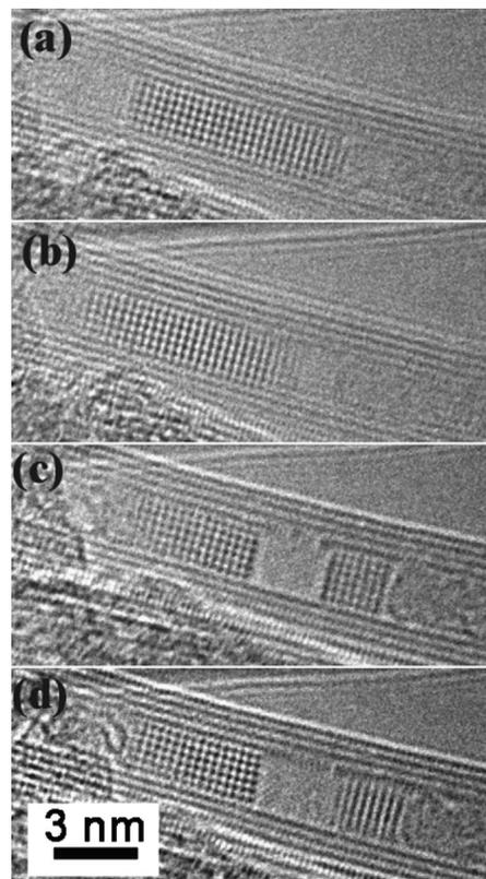
FIG. 1. HRTEM images of KCl nanocrystal(s) within a BNNT. The single KCl nanocrystal observed in (a) and (b) has been cleanly cleaved into two independent subunits, as seen in both (c) and (d).
