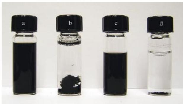
**Figure 2.** Photographs of vials containing a) a stable suspension of  $C_{18}\text{-}\alpha\text{-MM-SWNTs}$  in  $H_2O$  after more than three months, b) as-produced SWNTs in  $H_2O$ , which precipitate in several hours, c) stable suspension of  $C_{18}\text{-}\alpha\text{-MM-MWNTs}$  in  $H_2O$  after more than three months, d) as-produced MWNTs in  $H_2O$ , which precipitate over several hours.
