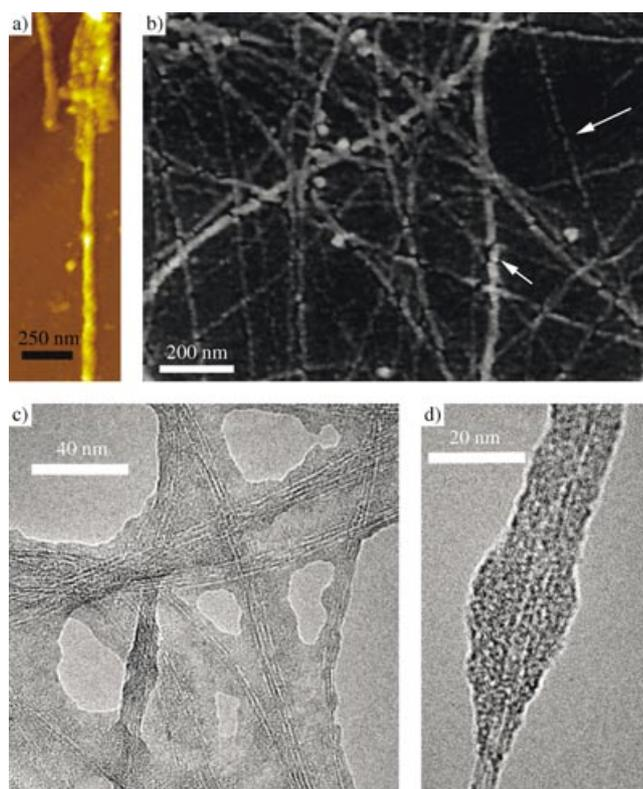
**Figure 3.** a) Tapping mode AFM image of  $C_{18}\text{-}\alpha\text{-MM-SWNTs}$  on a silicon substrate. b) SEM image of  $C_{18}\text{-}\alpha\text{-MM-SWNTs}$ . The arrows indicate damaged regions of the mucin mimic coating caused by the electron beam. c), d) TEM images of  $C_{18}\text{-}\alpha\text{-MM-SWNTs}$  stained with 0.5% methylamine vanadate.
