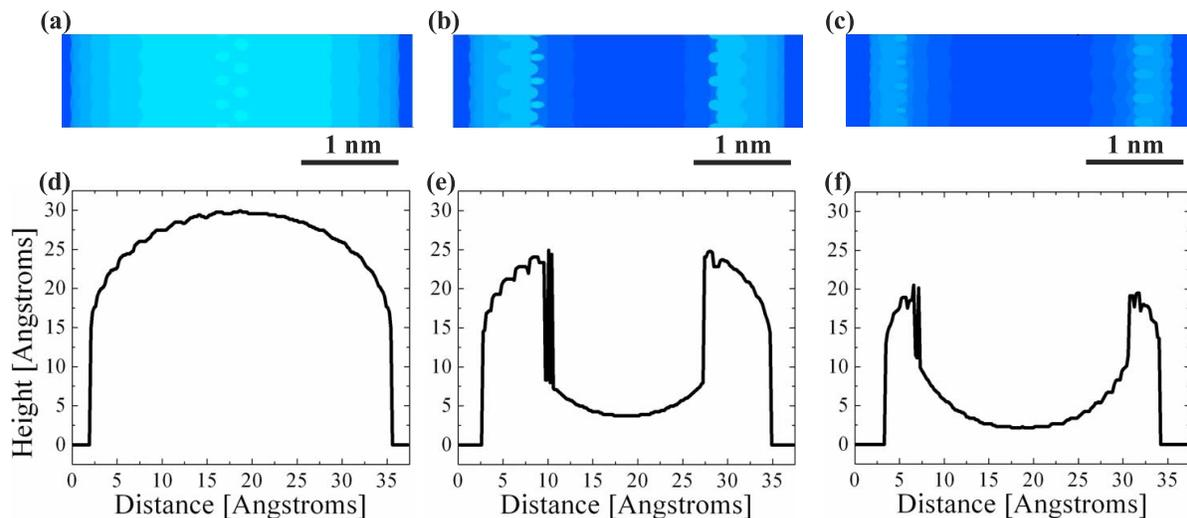
FIG. 2 (color online). Calculated STM images of a (20, 20) BNNT with (a)  $V_{\text{bias}} = -6.9$  V, (b)  $V_{\text{bias}} = -4.0$  V, and (c)  $V_{\text{bias}} = -2.1$  V. (d)–(f) are height cross sections for (a)–(c), respectively.
