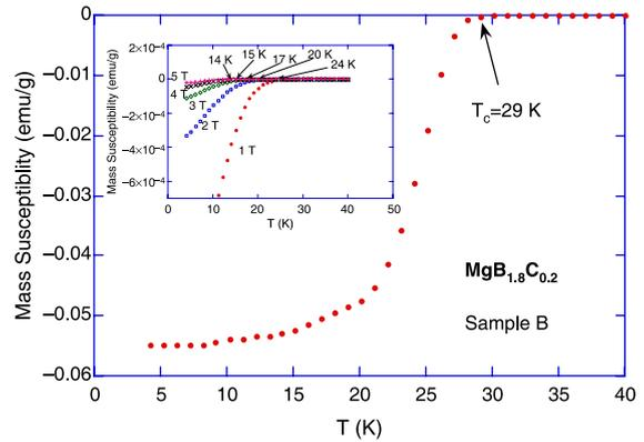
Fig. 2. Mass susceptibility vs. temperature for carbon-doped  $\text{MgB}_2$ , sample B, in a magnetic field of 100 Oe. Inset shows the onset transition temperatures at  $H=1, 2, 3, 4, 5 \text{ T}$ .
