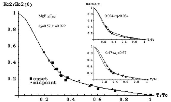
Fig. 5.  $H_{c2}/H_{c2}(0)$  vs. reduced temperature  $T/T_c$ . The data generated by the resistive midpoint criterion are plotted with triangles and those generated by the resistive onset criterion with squares. Also shown is the best theoretical fit. Due to the small spread in the data points, there are uncertainties in both parameters and they are shown in the insets.
