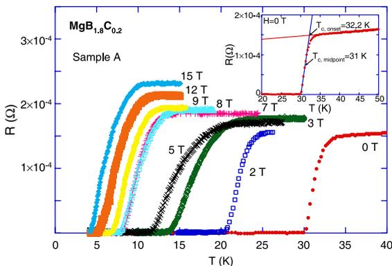
Fig. 1. Resistance vs. temperature measurements for carbon-doped  $\text{MgB}_2$ , sample A, at 0, 2, 3, 5, 7, 8, 9, 12, 15 T. The inset shows how  $T_c$  is determined by the resistive onset and midpoint criteria.
