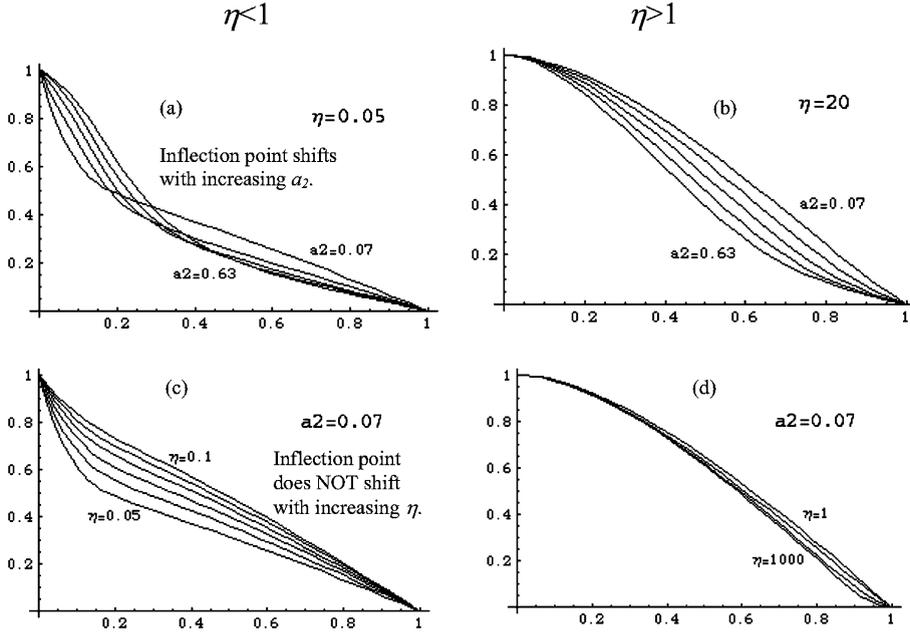
Fig. 4. Using Eq. (1) (see text), we explore how the shape of  $H_{c2}(T)$  for a dirty two-gap superconductor depends on  $a_2$  and  $\eta$ . We set  $\eta = 0.05 < 1$  in (a) and  $\eta = 20 > 1$  in (b) and plot  $H_{c2}/H_{c2}(0)$  vs.  $t = T/T_c$  for  $a_2 = 0.07, 0.21, 0.35, 0.49$  and  $0.63$ . We then set  $a_2 = 0.07$  and plot for  $\eta = 0.05, 0.06, 0.07, 0.08, 0.09$  and  $0.1 < 1$  in (c), and for  $\eta = 1, 10, 100$  and  $1000 \geq 1$  in (d).
