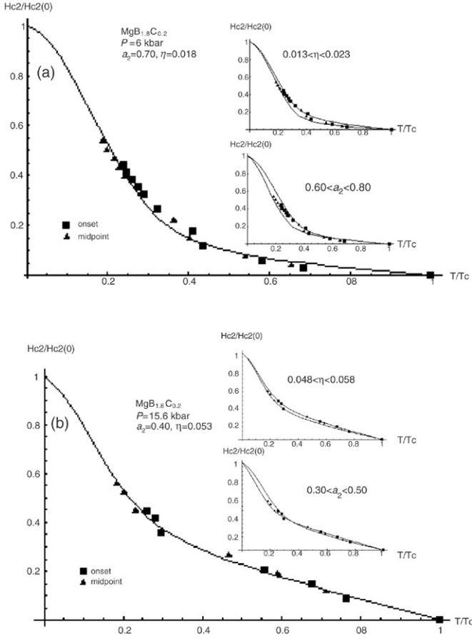
Fig. 4.  $H_{c2}/H_{c2}(0)$  vs. reduced temperature  $T/T_c$  at (a)  $P = 6$  kbar and (b)  $P = 15.6$  kbar. The data generated by the midpoint criterion are plotted with triangles and those by the onset criterion with squares. Also shown are the best theoretical fits. Due to the small spread in the data points, there are uncertainties in both  $\eta$  and  $a_2$  and they are shown in the insets.
