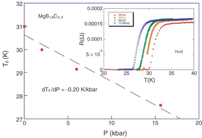
Fig. 1. Pressure dependence of  $T_c$ . The dashed line is a linear fit to the data,  $dT_c/dP = -0.20$  K/kbar. The inset shows  $R$  vs.  $T$  at  $P = 0, 2, 6$  and  $15.6$  kbar.
