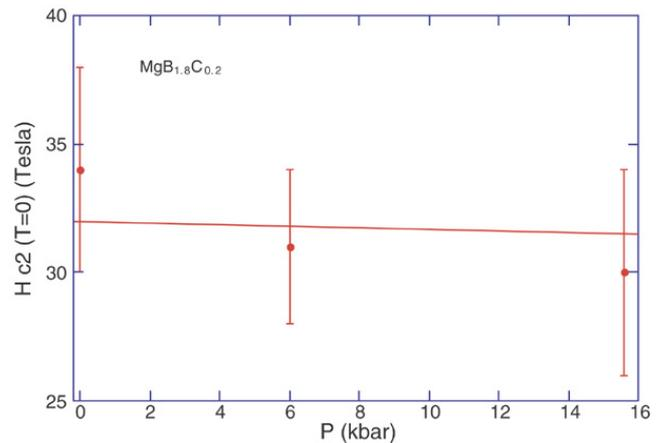
Fig. 3. The dependence of  $H_{c2}(T = 0)$  on pressure for  $MgB_{1.8}C_{0.2}$ . The error bars come from the difference between  $H_{c2}(T = 0)$  determined by the resistive midpoint and onset criteria. The result is consistent with the theoretical prediction for pure  $MgB_2$ ,  $dH_{c2}(T = 0)/dP = -0.036$  T/kbar [23], shown as a solid line.
