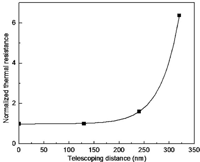
FIG. 4. Normalized thermal resistance  $R_T$  (inverse of  $K$ ) vs telescoping distance  $x$ . The error bar ( $\sim 3\%$ ) is less than the size of the symbol. The solid line is a fit to Eq. (1), with the characteristic electron localization length replaced by a phonon localization length  $l_{ph}=74$  nm.
