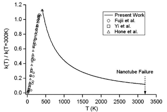
FIG. 3. Full temperature dependence of the thermal conductivity  $\kappa$  of MWNTs. Experimentally determined high-temperature  $\kappa$  reflecting umklapp and three-phonon processes [Eq. (2)] is plotted as a solid line. Also plotted are literature results for  $\kappa$  of various carbon nanotubes at low temperatures [15–17].
