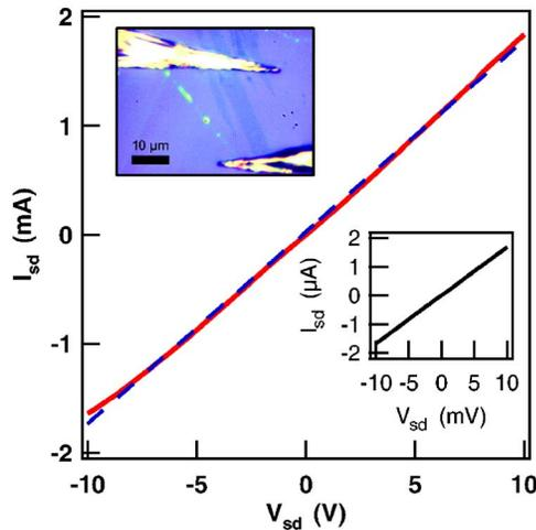
FIG. 2. (Color online) Source-drain current-voltage characteristic, with source-drain voltage  $V_{sd}$  in the range of  $\pm 10$  V, of the solder contacted graphene device shown in the inset, optical image (scale bar 10  $\mu\text{m}$ , image contrast enhanced). Dashed line is linear fit to resistance 5.7 k $\Omega$ . Inset plot is low-bias  $I$ - $V$  curve of same device, with a resistance of 6.0 k $\Omega$ . The back-gate voltage  $V_{bg}=0$  V.
