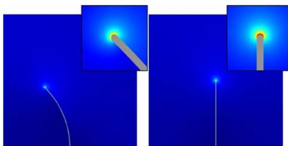
**Figure 3** Simulations of the electric field amplitude surrounds the nanotube when it is bent (left) and straight (right).
