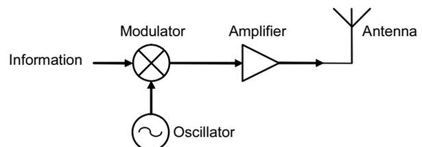
**Figure 1** Block diagram for a typical radio transmitter. The four essential components are the oscillator, modulator, amplifier and antenna.
