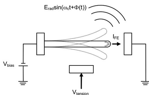
**Figure 2** Schematic of the nanotube radio transmitter. Field emission from the tip of the nanotube can induce self-oscillations in the nanotube. In combination with the excess charge in the tip of the nanotube, these mechanical oscillations effectively transmit a radio signal.
