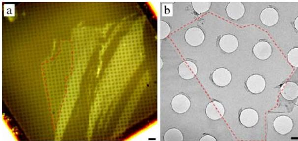
**Figure 1.** (a) Optical micrograph of graphene sheets on a perforated carbon film (c-flat, 1  $\mu\text{m}$  hole size), and (b) low magnification TEM view of a graphene sample. The single-layer regions are indicated by red dashed lines. Scale bars: (a) 2  $\mu\text{m}$ , (b) 500 nm.
