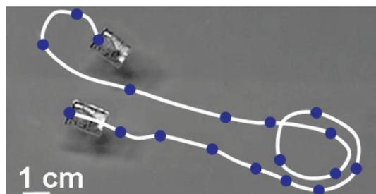
**Figure 4.** Light controlled linear motion of a VANT-PDMS composite floating on water. The top of the object has been colored black to aide the eye. The white line shows the path of the composite, with the dots representing two second time points. The composite is directed to the right, turned around in a circle, and sent back to the left. The final location of the boat has been superimposed upon the original image.
