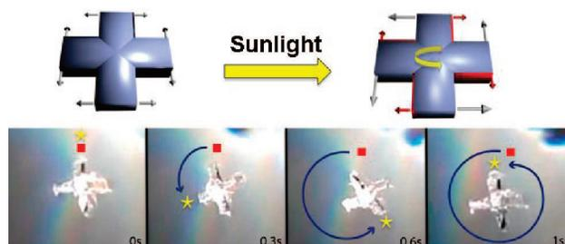
**Figure 5.** VANT-PDMS rotor timeline. Schematic (top) showing forces (gray arrows and with heating, red arrows) on PDMS rotor with absorbing material embedded on the clockwise face of each fin while dark and illuminated. Time line (bottom) of a VANT-PDMS rotor floating on deionized water with embedded VANTs on clockwise face of each fin and irradiated with focused sunlight. The square remains stationary as the star follows one fin.
