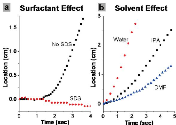
**Figure 2.** Location plots for a VANT-PDMS composite under constant, collimated laser illumination. (a) The quenching effect of the addition of the surfactant, SDS, on the motion of the composite. Illumination began at  $t \sim 1.3$  s. (b) Motion curve depicting the distance traveled by VANT-PDMS composites in water, IPA, or DMF filled troughs under nIR laser illumination, beginning at  $t \sim 0$  s.
