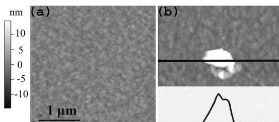
FIG. 3. Topographic map of the active layer of an organic solar cell device before (a) and after (b) forming a raised feature via C-AFM. The bottom part of (b) shows the height profile at the black line. The height of the feature is 60 nm.
