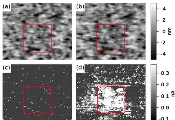
FIG. 2. (Color online) The  $1 \times 1 \mu\text{m}^2$  region outlined in red was scanned with a tip bias of 500 mV. Topographic maps of before (a) and after (b) reveal little change in the height profile, while the current maps before (c) and after (d) reveal a dramatic increase in conductivity.
