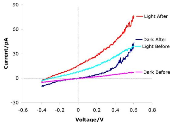
FIG. 4. (Color online) Current vs voltage response of the spot from Fig. 3 in dark and illuminated conditions before and after feature formation. Note that after the film has been locally current-injection treated, it exhibited much higher conductivity than before. The open circuit voltage increases from 0.29 to 0.33 V, and the short circuit current doubles from 7.6 pA before to 15 pA after.
