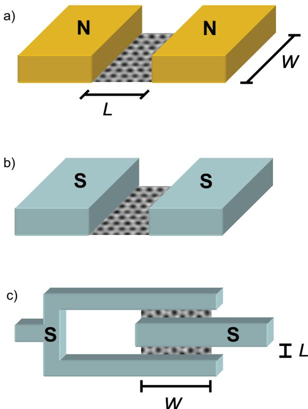
**Figure 1** (online color at: www.pss-b.com) Device geometries: (a) graphene sandwiched between two normal metal electrodes (N). The electrode spacing is  $L$  and the width of the graphene sheet is  $W$ . (b) Graphene Josephson junction with superconducting electrodes (S). (c) dc graphene superconducting interference device, as employed in Ref. [4]. The phase difference across the junctions is controlled by the magnetic flux through the loop A.
