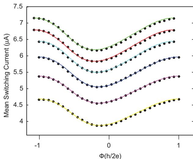
**Figure 3** (online color at: [www.pss-b.com](http://www.pss-b.com)) Measured mean switching current of a wide-and-short ( $W \gg L$ ) graphene dc superconducting quantum interference device as a function of magnetic flux. Traces are at different gate voltages, with  $-25$  V at the top, and spaced by  $10$  V. Overlaid are fits to the data described in the text.
