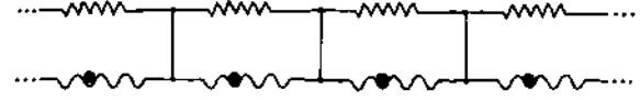
Fig. 2. Domain model for CDW conductor. The resistors represent normal electrons in parallel with charged CDW “particles” in periodic potentials. Carrier conversion is allowed by vertical shunts.
