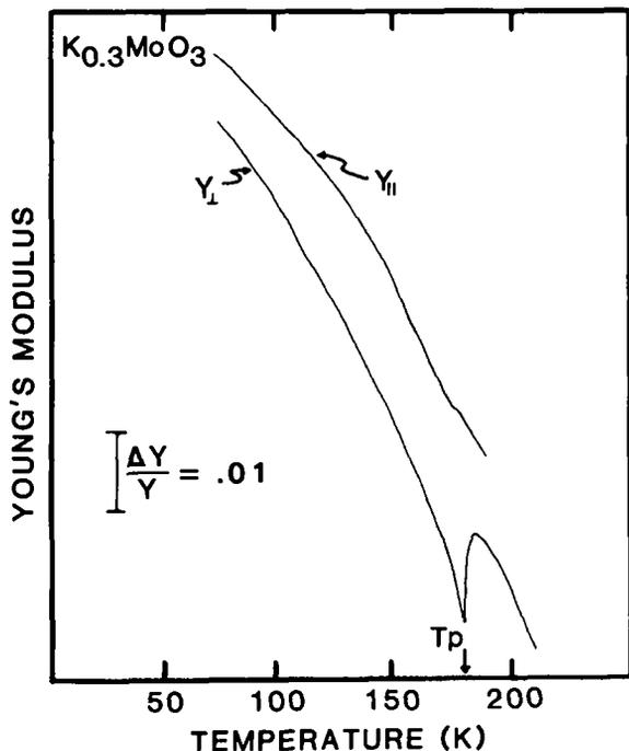
Fig. 1 Young's modulus  $Y$  measured both parallel and perpendicular to the  $b$  axis in  $K_{0.3}MoO_3$ . The data have been normalized to room temperature values. The vertical arrow identifies the Peierls transition temperature.
