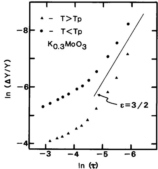
Fig. 4 Scaling behavior of  $Y_{\perp}$  near the Peierls transition temperature. The right-hand-most data points are 0.5 k from the transition temperature; the left-hand-most data points are 10 k from the transition. The sloping line is for a critical exponent of 3/2.
