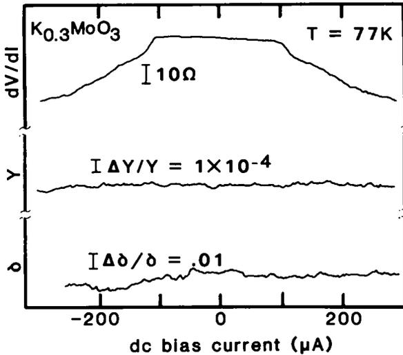
Fig. 3 Differential electrical resistance  $dv/dI$ , Young's modulus  $Y_{\parallel}$  and internal friction  $\delta$  in  $K_{0.3}MoO_3$ , as functions of dc bias current. CDW depinning has no effect on  $Y_{\parallel}$  or  $\delta$ .
