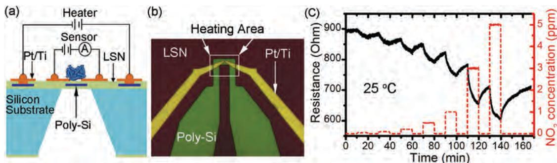
**Figure 4.** a) Cross-sectional schematic of the microheater sensor. b) Optical image of one microheater showing the Pt/Ti sensing electrodes above the polysilicon heater. c) Real time response of the sensor at room temperature toward different NO<sub>2</sub> concentrations.
