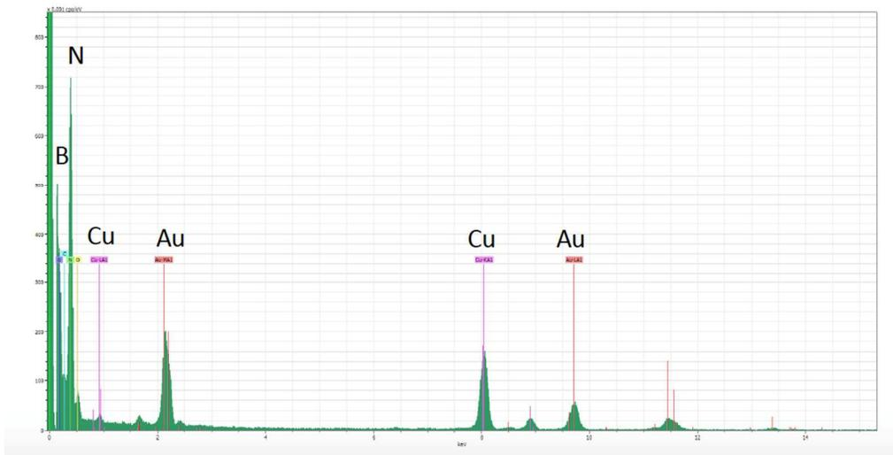
**Figure S2.** HAADF image and EDS spectrum of a Au nanorod within a BNNT showing only Au signals with negligible trace of O and Cl. Cu peaks in the spectrum are from the
