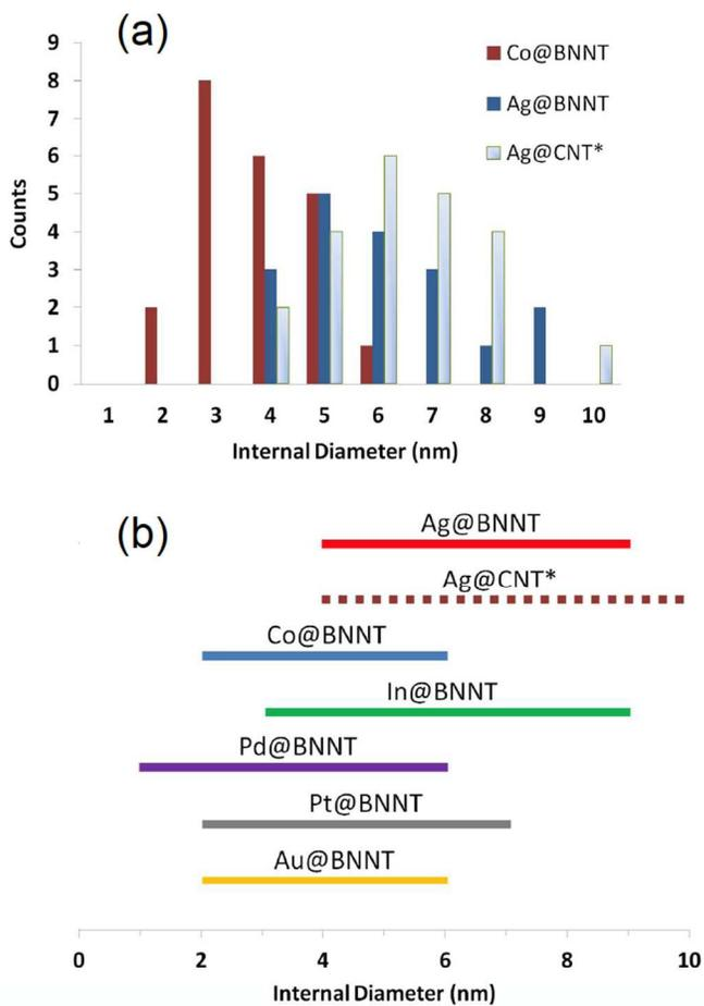
**Figure S4.** (a) Histogram of the diameter distribution of the internal cavity of BNNTs encapsulating Co and Ag. (b) Typical ranges of internal cavity diameters of BNNTs containing various filling metals. For comparison, the distribution and diameter ranges for Ag within CNTs (denoted Ag@CNT\*) is taken from Ref. 32.
