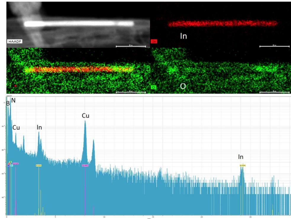
**Figure S3.** HAADF image, EDS mapping and EELS spectrum of In@BNNT. Indium oxide is indicated at the two ends of In nanorods. This suggests that pure In nanorods were initially formed and subsequently oxidized in the presence of either ambient oxygen or resultant products of the salt reduction inside the BNNT after thermal reduction was carried out. Cu peaks in EELS spectrum originate from the copper TEM grid.
