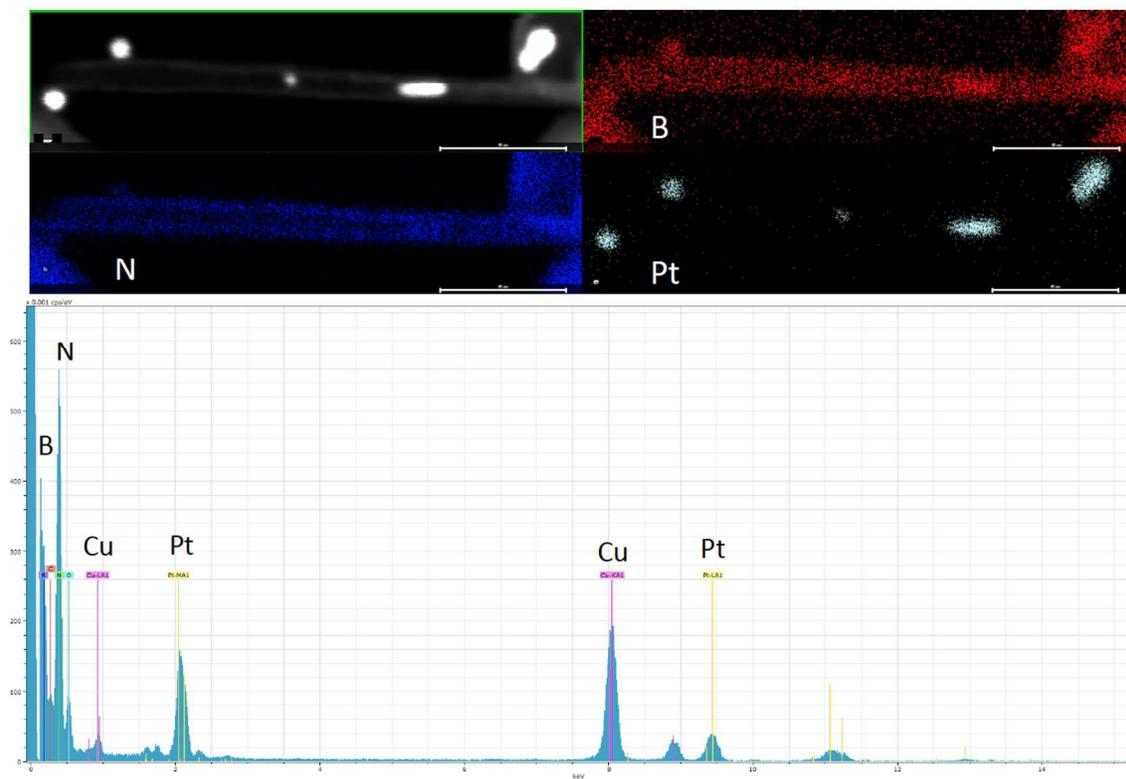
**Figure S1.** HAADF image, and EDS mapping and spectrum of Pt@BNNT. Cu peaks in EDS spectrum are from the copper TEM grid.
