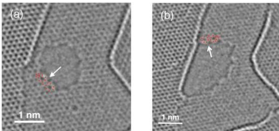
Figure SI5. Topographic defects (pentagon-heptagon (5|7) pairs) at the defect edge in h-BN (at 900 °C). Red dots illustrate atom positions and white arrows indicate topographic defects.
