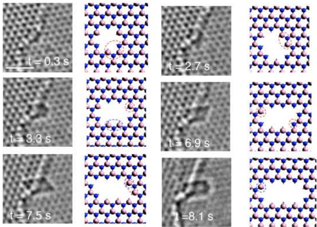
Figure SI3. Time evolution of atomic structure of a hexagon defect at 900 °C. The red dotted circle indicates atom or chain of atoms, which will be removed in the next time frame while the blue circle indicates newly added atom(s). Scale bars are 1 nm.
