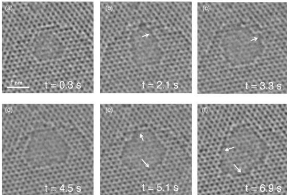
Figure SI4. HRTEM images of a hexagon defect at 900 °C. The white arrows indicate bundles of atoms, which were ejected while the defect grows.
