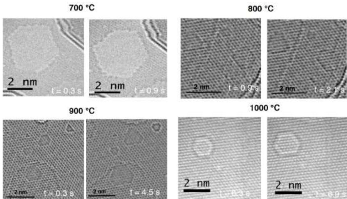
Figure SI2. HRTEM images of hexagonal defects at 700, 800, 900 and 1000°C. The time label in each image indicates when they were taken in a particular fixed-temperature time-series.
