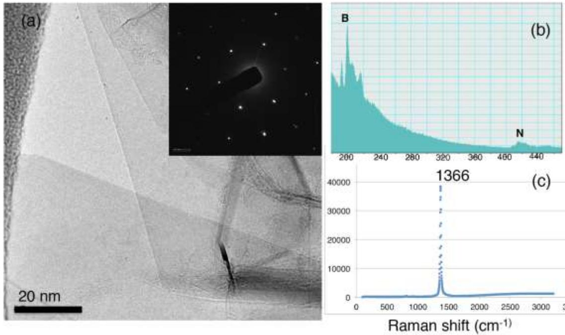
Figure S11. (a) A TEM image of as – prepared h-BN flakes. (Inset) Selected area electron diffraction shows high crystallinity of our materials. (b) EELS and (c) Raman spectrum confirm the chemical composition of our h-BN.
